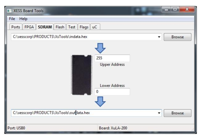
The serial flash can be handled in the same manner as the SDRAM by using the *Flash* tab. The only additional feature is that the flash can be loaded with an FPGA configuration bitstream by entering a *.bit* file into the upper text field.
