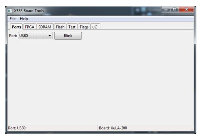
The FPGA tab is used to download configuration bitstream files into the FPGA. You can select a bitstream file by:
