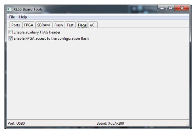
The microcontroller can be reprogrammed by entering the name of an Intel HEX file into the text field of the uC tab and clicking on the downward-pointing arrow.
